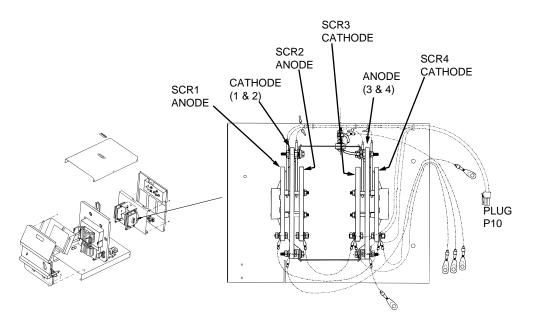
FIGURE F.14 - SCR TEST POINTS.
